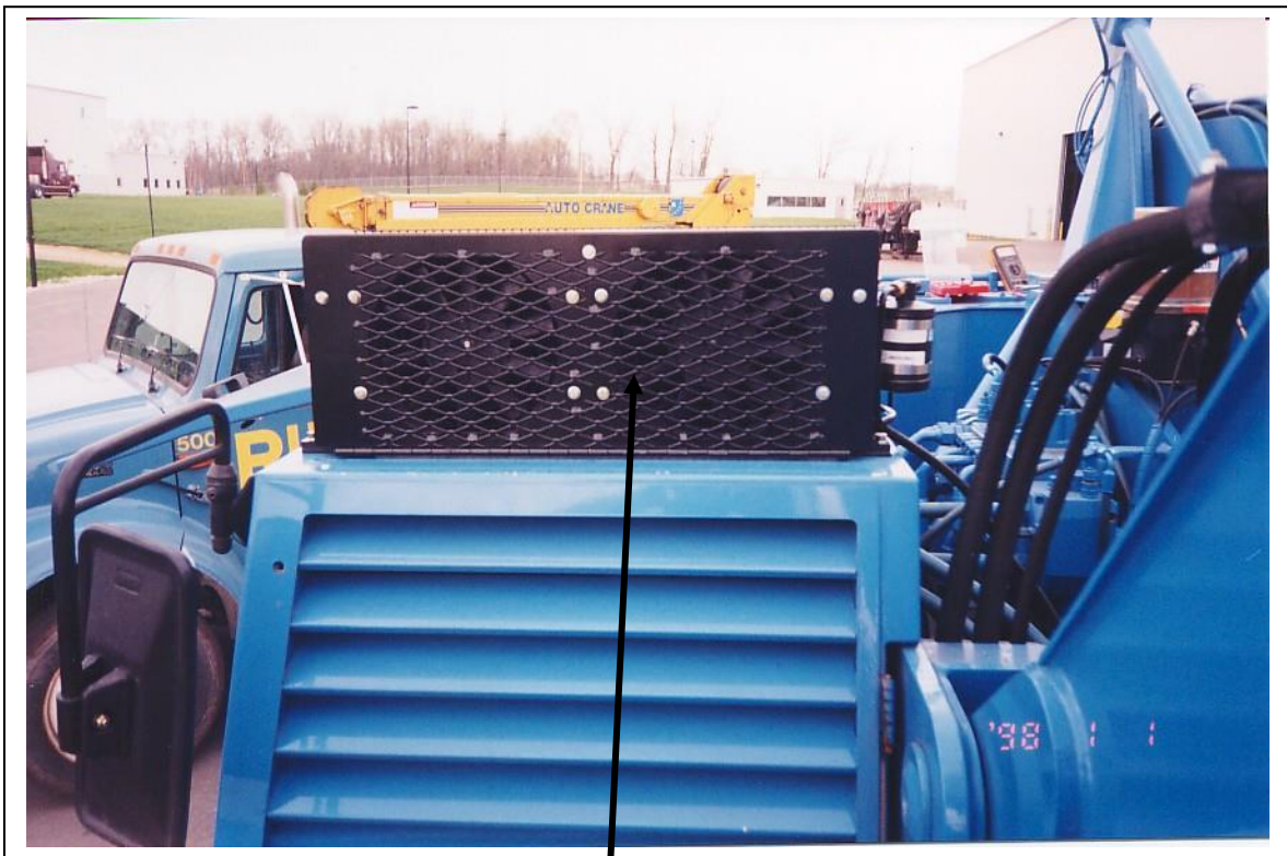
3/8" bolt up through bottom of radiator shroud.
